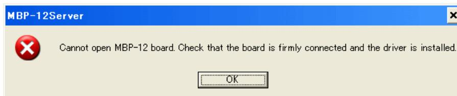
If an error message is displayed, check if **VBF2008** exists in **Sound, video and game controllers** in **Device Manager**. If it does not exist, check the connection of the MBP-1244 board and installation status of the driver.
