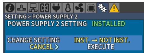
To change Power Supply 2 installation status, turn CONTROL, select EXECUTE in the CHANGE SETTING Menu and press CONTROL.
