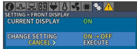
\* Menu Display Settings before turning off the power are retained when re-starting the unit.
