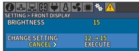
The Menu display contrast can also be adjusted following the above procedure but by selecting **CONTRAST**.
