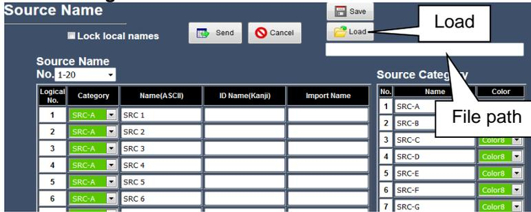
Enter the file path in the field and click the **Load** button to load the saved settings.
