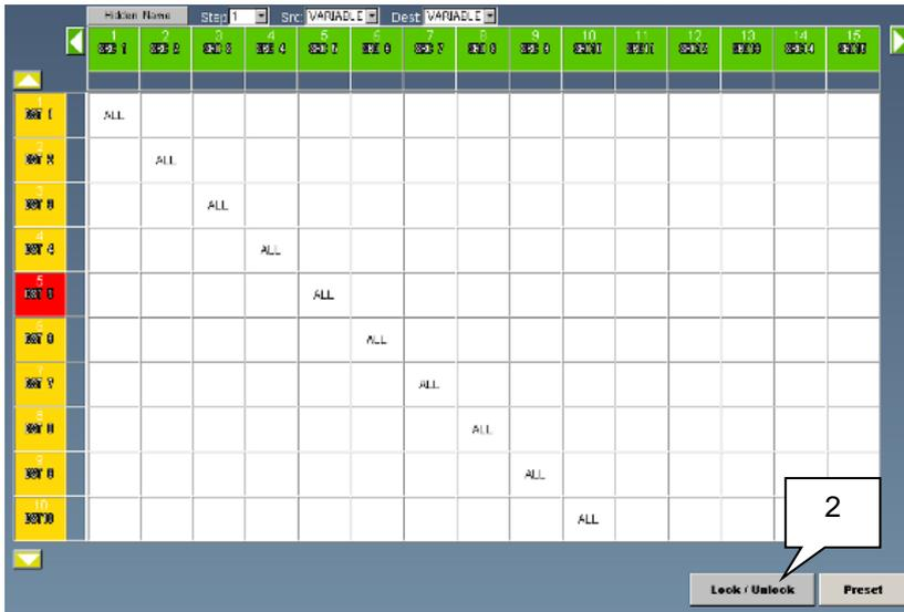
To verify the Lock All status, move the mouse over destination buttons. "Lock All: Locked" is displayed if a destination is set to LOCK ALL.
