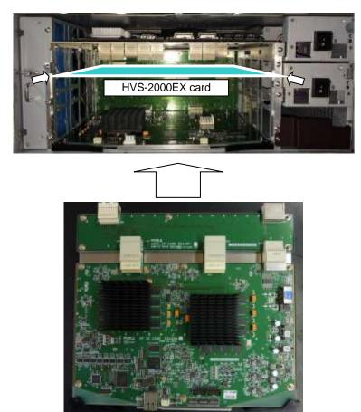
(3) Tighten the two screws at both sides to secure the front panel to the chassis.
