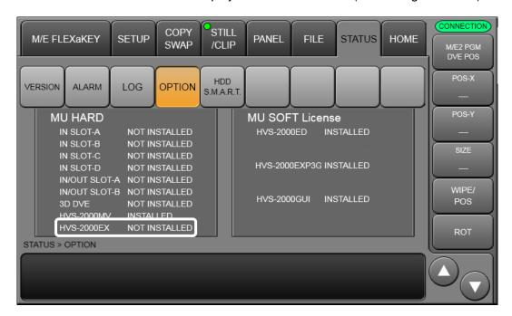
(2) Verify that the HVS-2000EX card functions properly. Check that advanced chromakey channels are available. Check that additional Color Corrector channels are available. Refer to the HVS-2000/OU Operation Manual for more details.
