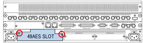
(3) Align the HVS-49AES card with the slot guide rails and carefully slide the card into the slot.
