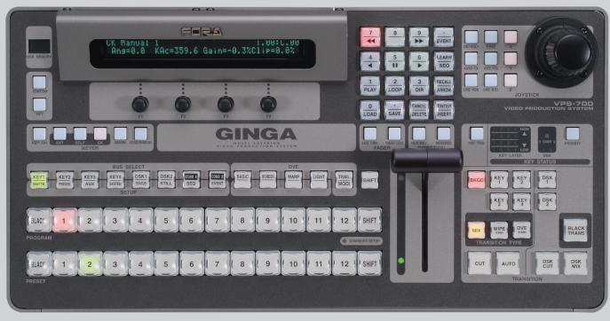
The compact and easy-to-use control panel of the VPS-700 has basic PGM/PST rows and fader levels, 3-axis joystick, parameter display, and optional touch panel controller. Despite these numerous ground-breaking functions, the VPS-700 will not overwhelm you with complicated operations.
