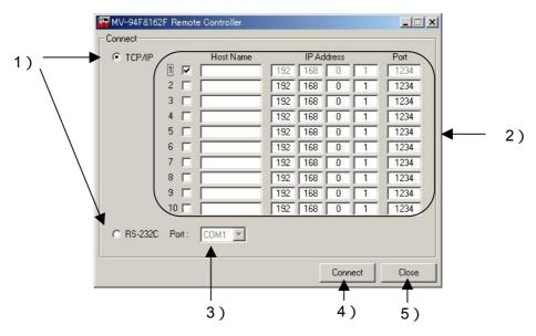
1) Connection method select button (TCP/IP, RS-232C)
