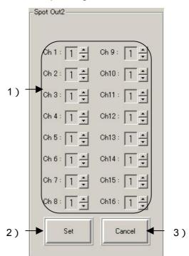
Video auto sequencing interval Used to set the sequencing interval of each video during auto sequencing. Set the interval between 0 and 30 seconds. Videos with sequencing intervals set to 0 sec. are skipped during auto sequencing.
