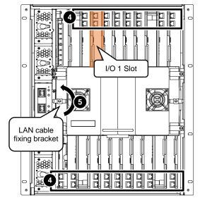
(6) Loosen the four fixing screws at the four corners of the front card unit, and pull the front card unit straight out toward you.
