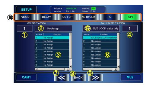
The current input pin assignments are displayed in ③. The current output pin assignments are displayed in ⑥.
