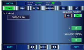
4) Turn the top left knob and select a TV standard, then press the knob to confirm the selection. The massage "Do you want to change video format?" appears. Select OK. Then the TV standard will be changed.
