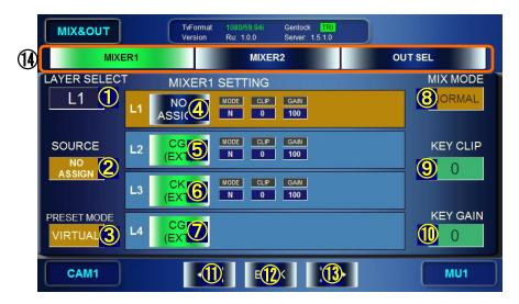
①②③ Select a layer mode at ③. If USER1, 2 or 3 is selected, select a layer at ① and its video source at ②.
