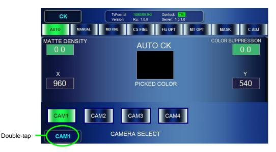
To change the camera selection, tap a button among **CAM1** through **CAM4**. The selected button turns green, and the indication on theCamera selection button changes to the selected camera.
