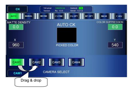
3) Once a camera is dropped on another camera, the CAMERA COPY menu as shown below appears] Verify that the source and destination cameras are properly set. The source and destination cameras can be changed in this menu. Tap ACCEPT to perform the parameter copy. Tapping CANCEL cancels the process.
