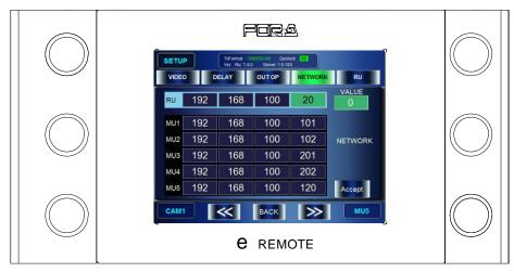
a) Turn the knob at top left, or tap a box of digits to select a box in RU IP address which you are going to change the value of. (The selected box turns to green.)
