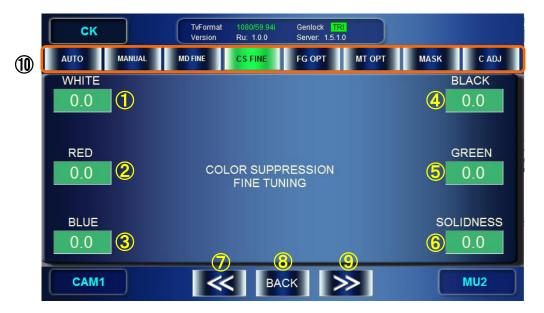
$(\ensuremath{\underline{1}})$  to  $(\ensuremath{\underline{6}})$  Adjust the suppression of backing color on the foreground images where white component is included.
